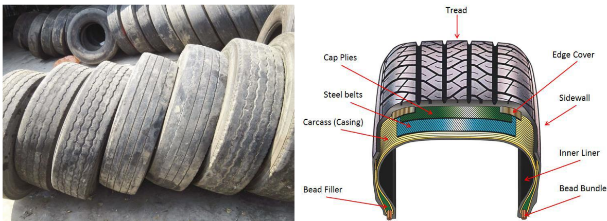
Figure 14 Disposed car tyres (Left); tyre schematics (Right)
